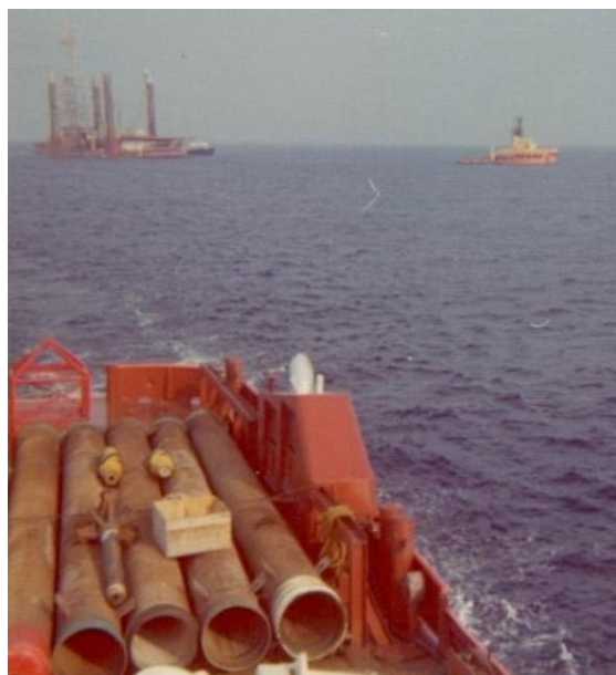
On the Northern Builder with 30 inch casing on deck, in the background a rig is being shifted by an 8000hp tug
