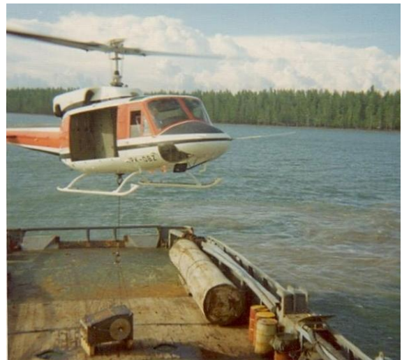
Loading a heavy mud pump from the airport at Tarakan, Note helicopter doors stripped off to lighten the weight of it
