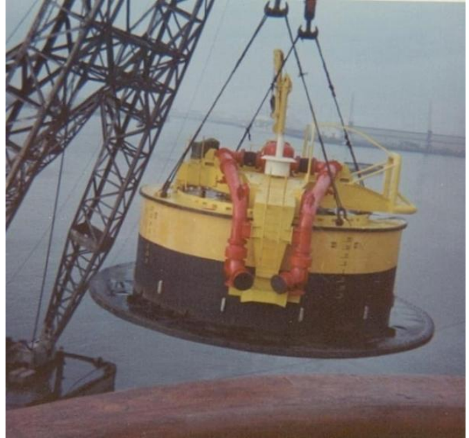
Above - 11 January 1970 in Rotterdam - Loaded a 177 ton single point buoy for use off the Bluff in Durban, discharged into the harbour in Durban using the ship's heavy lift derricks.
